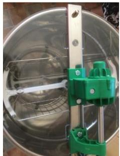
This shows the bar carrying the rotation gearing. Note the 13mm nut, of two, holding the bar in position. These have to be removed to dismantle the machinery for cleaning. **Not to be lost!**
