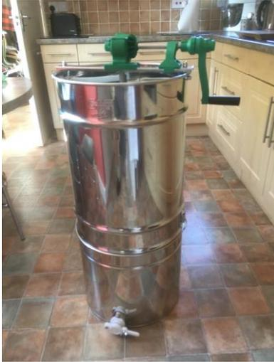
The extractor stands firmly and conveniently on the floor of the kitchen. It is manually operated. Below the extractor drum and attached by easy clips is a sump which acts as a collecting and settling tank. It holds around 50lb of honey. About two good supers worth. Honey runs during the extracting through holes in the floor between the two drums. It passes through a built-in, removable filter and into the lower drum.
