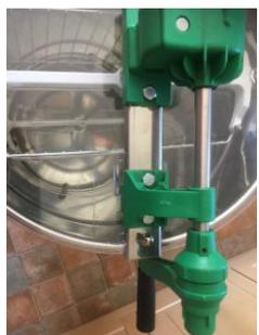
This is the handle showing the spring loaded Clutch mechanism which allows the extractor to free-wheel. Note the two ridges in line which have to be in position for the clutch to engage.
