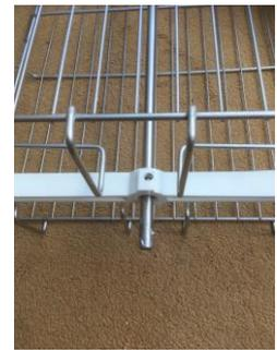
The spindle bearing end to be greased
