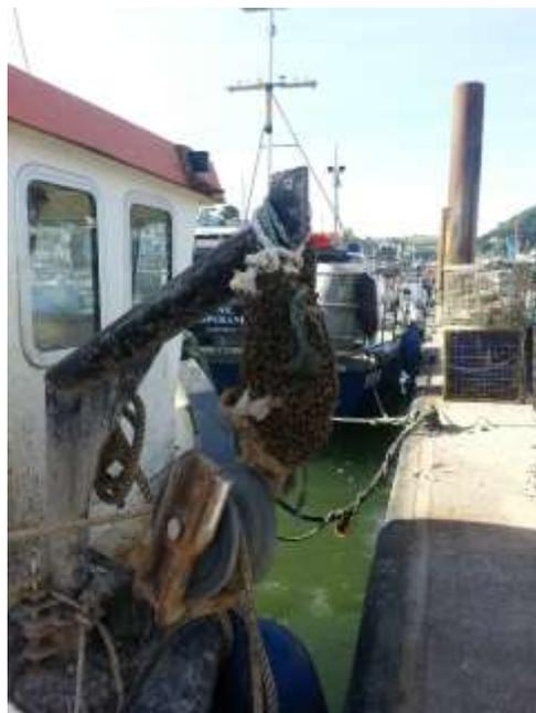
The equipment they decided to hang onto, is a part of the winch hauling system, which serves to pull the crab pots up from the sea floor by means of a small rope which is firstly put onto the open pulley at the end of the arm (below where the bees are clinging) and from there to the winch drum, which would be spinning to put tension on the rope and so, bring the crab pots to the surface of the water.
